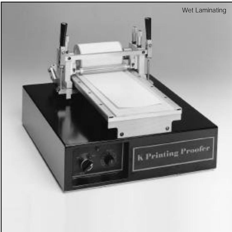
Both wet and dry laminated samples can be produced on the machine using the gravure head with K-Lam laminating accessories. These accessories include a rubber covered bed and wired K-Lam bars which are fitted in place of the doctor blade assembly to control adhesive coating weight.
